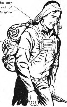
Tie here and provide shroudline loops for adjusting
